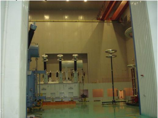
2. Frequency test transformer YDTW-600/300
