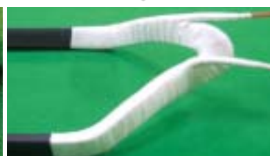
End Section of Coil Taped Manually
