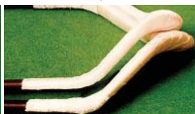
Coil Insulated with MICA Tape
